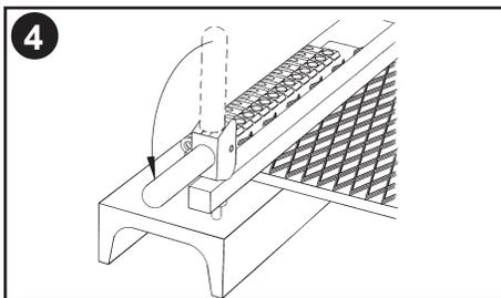
4. Clamp belt securely. (NOTE: Clamp levers are adjustable.)
