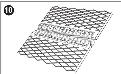
10. Notch trailing edge of belt on both sides. Bring belt ends together and insert hinge pin. Bend the opposite pin side so that both ends are bent in the same direction and pin will not fall out. Remove nails from the tool.
