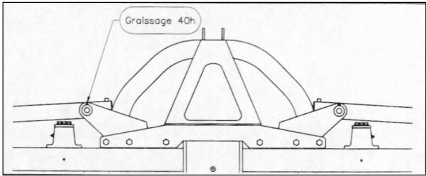
Figure 36 : Cylinder yokes
