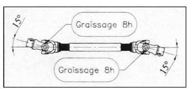
Lubricate locks jaw and coat the sliding tubes of Lithium base grease EP-2 every 40 hours
