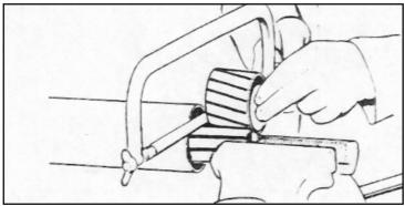
Figure 18 : cutting of the metal shaft
