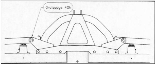
Figure 36 : Cylinder yokes
