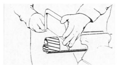
Figure 17: Cutting the plastic
