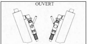
Figure 24 : unlocking the folding cylinders
