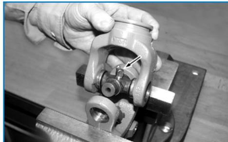
When mounting second yoke, make sure that grease zerk is easily accessible (arrow).
