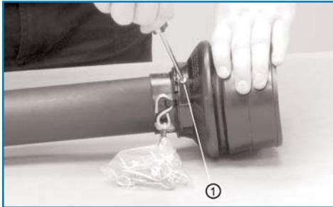
Remove locking screw from new replacement shield **(1)**. Retain screw for use in later step.
