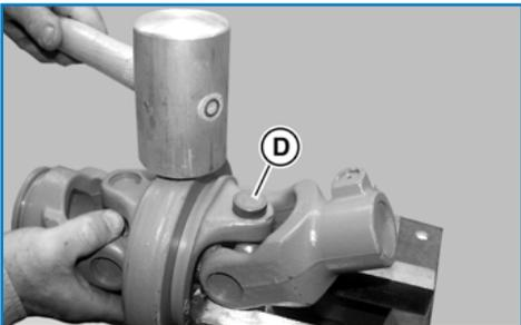
Position yoke as shown and use light hammer blows to drive out needle bearing cap **(D)**.
