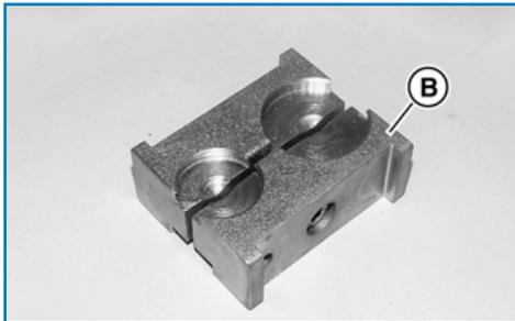
Dismantling tool Part# 4000001 **(B)** compatible only for cross and bearing kits Walterscheid Series 2300/2400/2500/2600, Agmaster Series 3/4/5, and Bondioli equivalent style S4.
