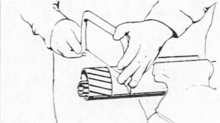
**Figure 17: Cutting the plastic**
