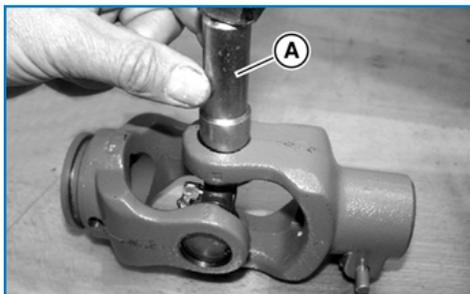
Relieve snap rings of stress with hammer blows to the drift punch Part# 4000004 (**A**).
