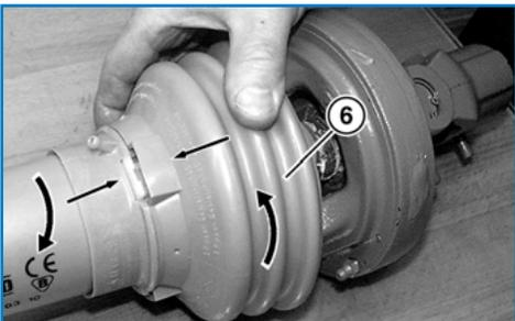
Rotate cone to mounting position where bearing ring tabs align with notches in the cone (arrows).
