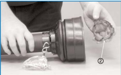
Remove the new shield bearing ring **(2)**. Retain for use in later step.
