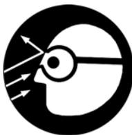
To reduce the risk of injury to your eyes never operate a **107 DRILL** unless wearing goggles or properly fitted safety glasses with adequate top and side protection.
