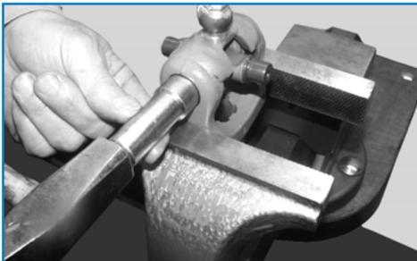
Drive in new needle bearing cap using drift punch Part# 4000004, until snap ring groove is visible.
