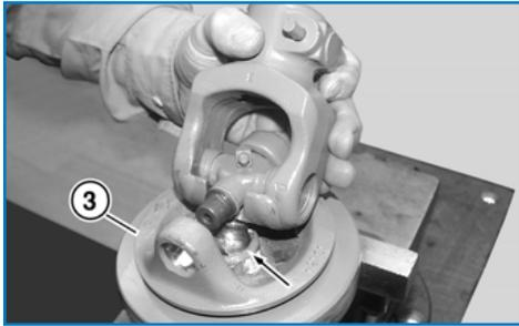
Grease guiding parts (arrow) with a white grease paste. (We recommend Gleitmo 810 or similar).
