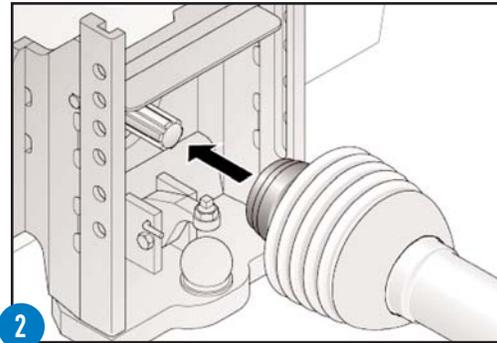
2 Slide PTO drive shaft onto tractor power take-off shaft until lock engages automatically.
