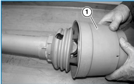
Remove and discard original double-yoke guard cone **(1)**.
