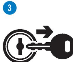
Prior to maintenance and repair work, switch off the engine, remove the ignition key and wait until all moving parts of the machine have come to a complete stop.
