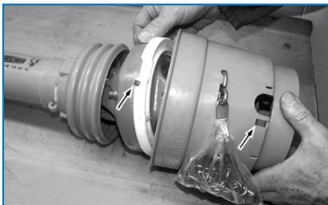
Slide new guard cone for the CV double yoke from the connecting end over the tab of the bearing ring. Ensure the holes for the screws are visible in the slots.
