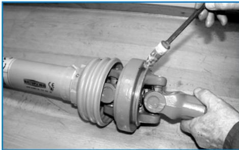
Grease bearing groove on the CV double yoke.
