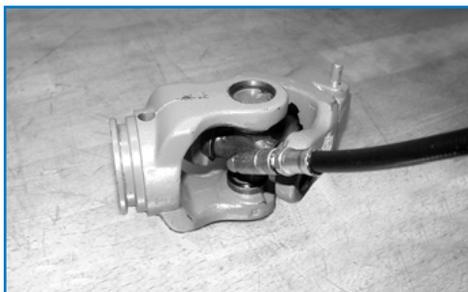
Grease joint until grease escapes from seal.
