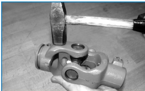
Relieve joint of stress by applying hammer blows to yoke ears.
