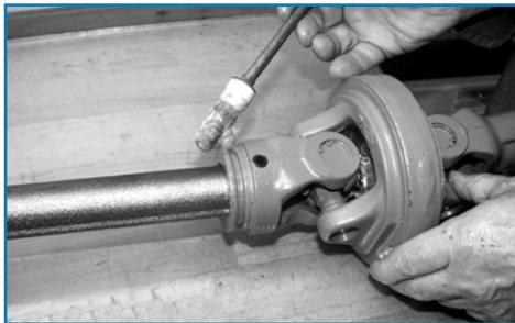
Grease the inner profile tube and the bearing groove on the yoke.
