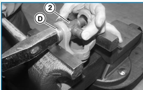
Insert cross **(2)** into yoke. Use cross journals to guide bearing needles when inserting needle bearing cap **(D)**.
