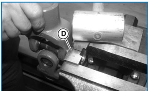
Depending on the size and style, where compatible, we recommend using special tool Part# 4000001 or 4000003 (B or C) to clamp the needle bearing cap (**D**). With or without the special tools, remove needle bearing cap with light hammer blows on the yoke or by turning. Caution: Do not deform the yoke ears or strike the bearing cap.
