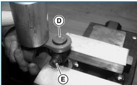
Rest cross journal **(E)** on protected vice jaws as shown and drive needle bearing cap **(D)** up with light hammer blows. Remove and discard original needle bearing cap as described above.
