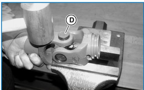
Position joint as shown and use light hammer blows on yoke to drive out needle bearing cap (**D**).
