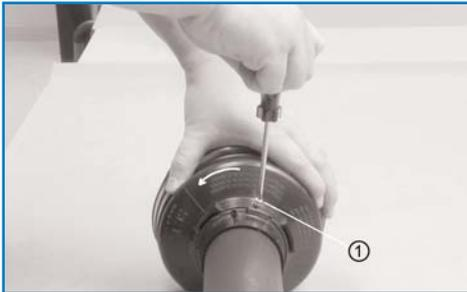
Rotate cone to locking position where a bearing ring tab aligns with the screw hole (arrows).
