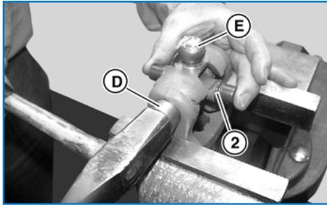
Insert cross **(2)** into yoke with bridge **(E)**.
