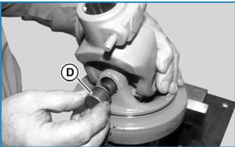
Attach the needle bearing cap **(D)** and drive in. When driving in the needle bearing cap, guide the bearing needles with the cross journal. Drive in needle bearing cap using drift punch Part# 4000004 until snap ring groove is visible.
