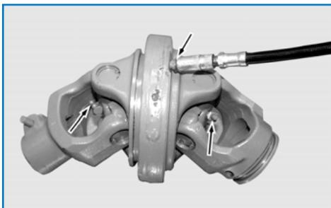
Grease the joints and double yoke until grease escapes.
