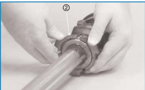
Place new bearing ring **(2)** on the bearing groove with tabs facing profile tube.
