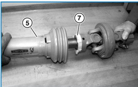
Place new bearing ring **(7)** on the bearing groove with tabs facing profile tube. Slide on the new half-shield **(5)** over the profile tube.
