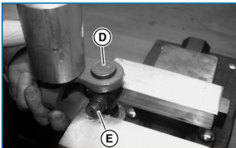
Rest cross journal **(E)** on protected vice jaws as shown and drive needle bearing cap **(D)** out with light hammer blows. Remove and discard needle bearing cap and the cross.
