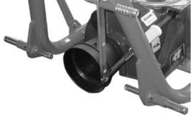
The machine must be positioned, through the raising of the lower connections of the tractor, so that the land distance from the lower extremity of the pendulum is approximately of 75 cm.
