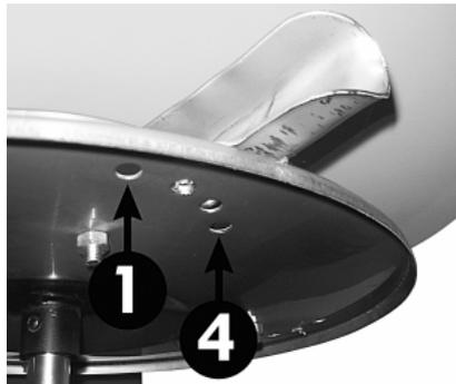
*Spreading disc's vanes regulation*
