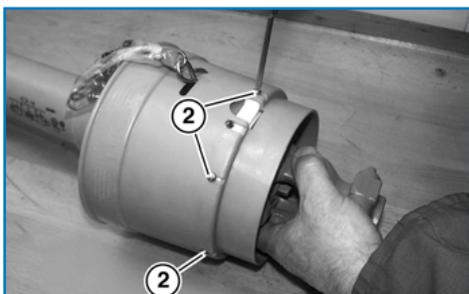
Install the new fastening screws **(2)**.
