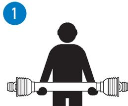
Keep the driveline horizontal during handling to reduce the risk of an accident due to the driveline sliding apart.
