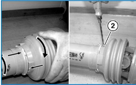
Rotate cone to locking position where a bearing ring tab aligns with the screw holes.
