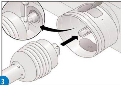
3 Slide PTO drive shaft onto the implement/machine point of implement connection and securely lock.
