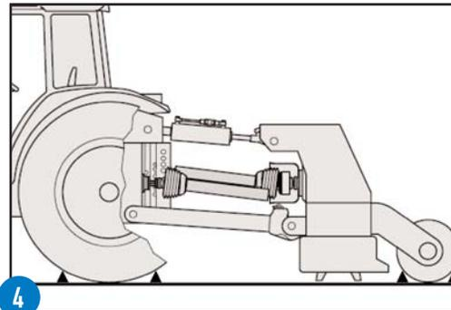
4 For length adjustment, hold PTO drive shaft halves next to each other in shortest operating position.
