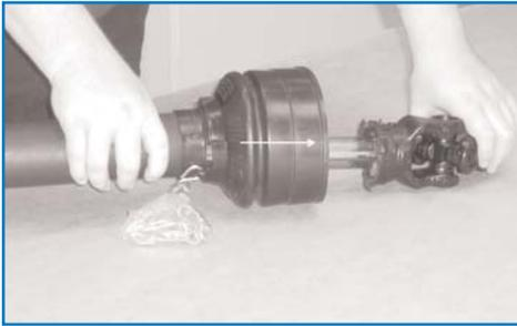
Slide on the new half-shield over the profile tube (arrow).
