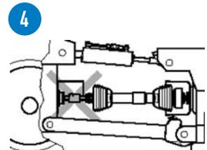
Do not use spline extensions or adapters on the tractor PTO Shaft.
