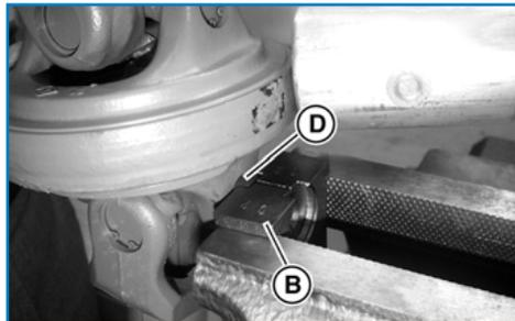
We recommend clamping the yoke and needle bearing cap **(D)** in special tool Part# 4000001 or 4000003 **(B)** or **(C)**. Continue to remove needle bearing cap by light hammer blows on flange or by turning assembly.
