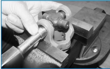
Drive in needle bearing cap using drift punch Part# 4000004, until snap ring groove is visible.
